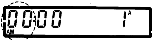
Leak Detect Mode "Disable" Display
